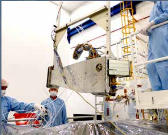
SPICE Optics Unit being assembled on to the Solar Orbiter spacecraft. Credit: Airbus DS
