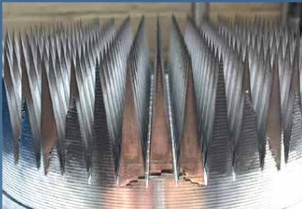
Black body calibration target former for MetOp-SG. Credit: STFC RAL Space
