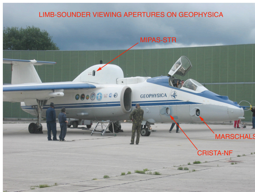
Figure 9 Location of MARSCHALS, CRISTA-NF & MIPAS-STR on the Geophysica
