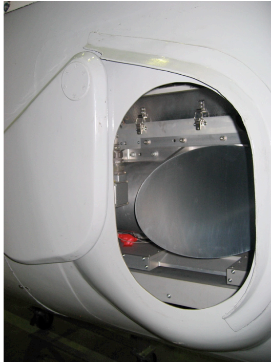
Figure 4 MARSCHALS Antenna seen through the open aircraft aperture
