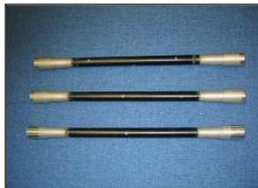
CFRP truss structure
