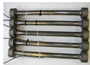
TiSiC truss structure
