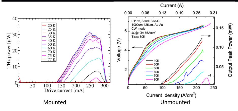
Block integration concept works! Minimal change in threshold current or maximum operating temperature.
