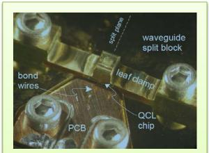
QCL + waveguide + horn antenna
