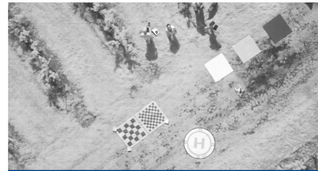
Raw Calibration image from the Near-Infrared imager of the RAL Space hyperspectral system. Credit: STFC RAL Space
