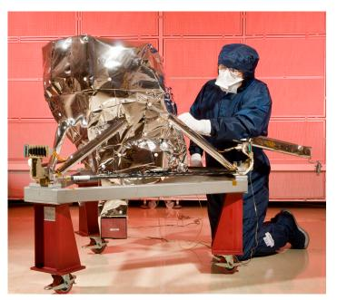
The foil and netting design is hugely effective, making thin gaps in between the foils where the netting doesn't allow it to touch – preventing heat from being conducted from one layer to another. There is no air in space so heat can't convect between the layers, and the surfaces are shiny to restrict the amount of heat that is radiated.
