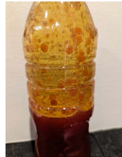
Gas bubbles carry water bubbles up through the oil. When the gas bubble pops, the water bubble falls back down.
