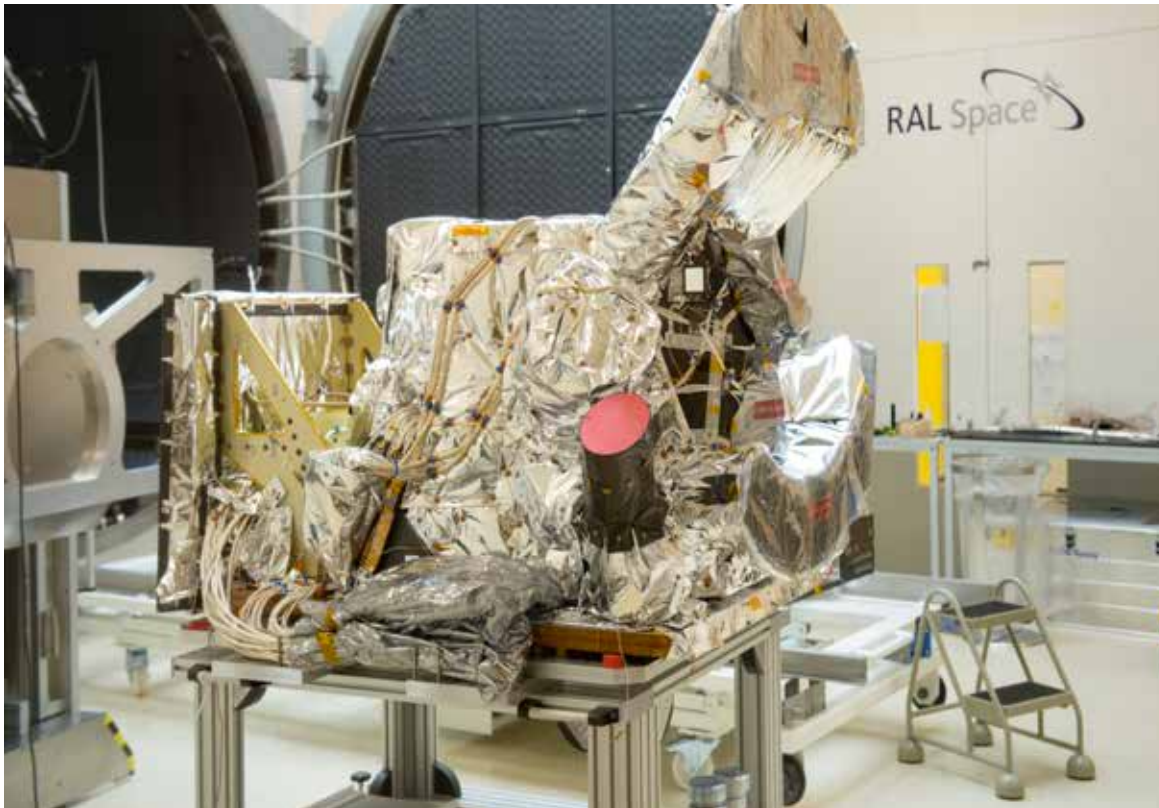
SLSTR undergoes calibration testing in the UKCCSI
